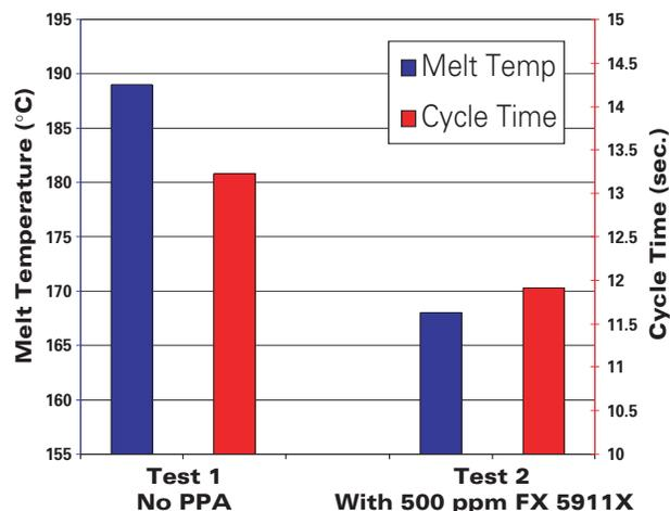
This graph shows the melt temperature and the corresponding cycle time. Test 1 is at the start of the experiment, before PPA was added. Test 2 corresponds with the final parameters after the PPA was added. The addition of 500 ppm of FX 5911 allowed for a reduction in the extrusion temperature. The resulting lower melt temperature allowed for a decrease in the process cycle time because cooling time could be shortened.
