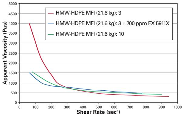
**Capillary Rheometry: T= 220°C, capillary diameter=2 mm, L/D 15**
