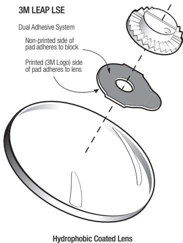
**3M LEAP – Designed for Automated Edging Machines** uses the same technology as LEAP, however, is formatted for robotic pick up with precision pad placement. Consists of larger roll sizes, for fewer change outs; a double liner, and feed line for easy thread up.
