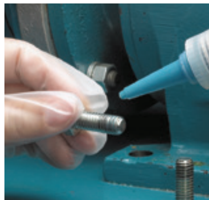
Adhere and seal threaded assemblies: 3M™ Scotch-Weld™ Threadlockers (pg 24-25 )
