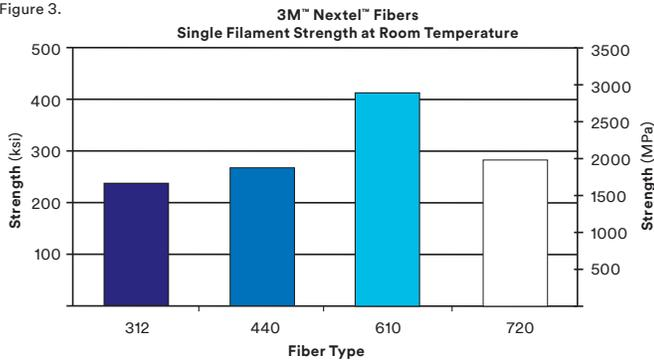
Test Description: Extension Rate: 0.2 inch/min (5.1 mm/min)
