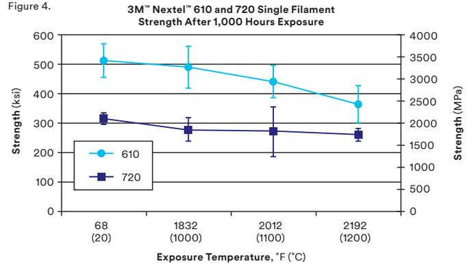
Outline of Test: Crosshead Speed: 0.02 inch/min (0.5 mm/min)
