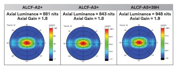
**Note:** Samples measured on a 12.3" IPS display with White Reflector/Light Guide/Diffuser/BEF3-t-155n/ALCF-AX+ film stack Axial Gain with reference diffuser only.
