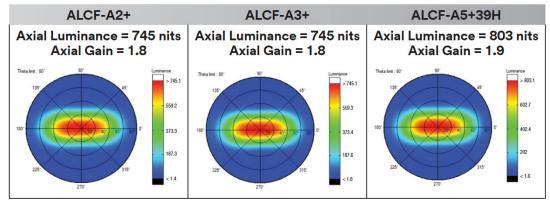
**Note:** Samples measured on a 12.3" IPS display with White Reflector/Light Guide/Diffuser/BEF3-t-155n/ALCF-AX+ film stack Axial Gain with reference diffuser only.
