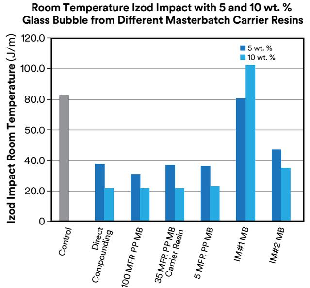
Figure 7. Room Temperature Izod Impact Changes with Different Masterbatch Carrier Resins
