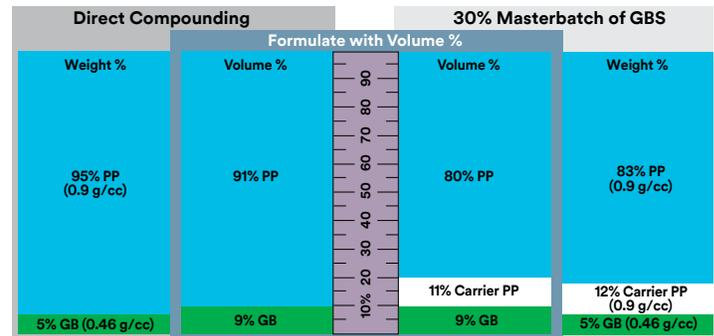
Figure 1. Directly Compounded 5% 3M™ Glass Bubbles vs. Masterbatch Addition of 3M™ Glass Bubbles – Carrier Resin wt. and Vol. % Implications.
