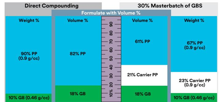
Figure 2. Directly Compounded 10% 3M™ Glass Bubbles vs. Masterbatch Addition of 3M™ Glass Bubbles – Carrier Resin wt. and Vol. % Implications.
