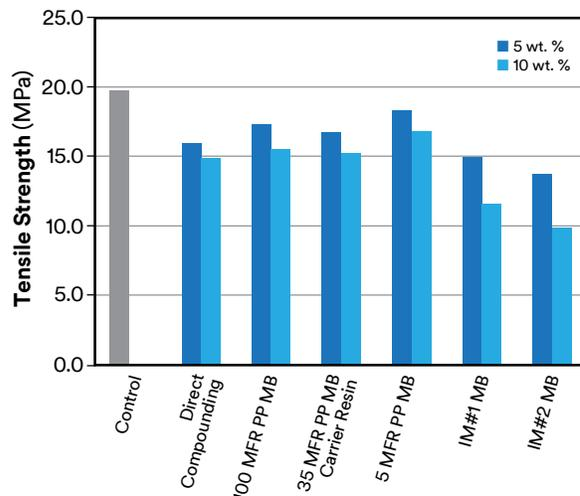
**Figure 3.** Tensile Strength Retention with Different Masterbatch Carrier Resins
