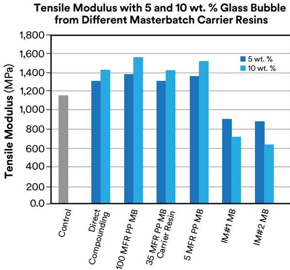
Figure 5. Tensile Modulus Changes with Different Masterbatch Carrier Resins
