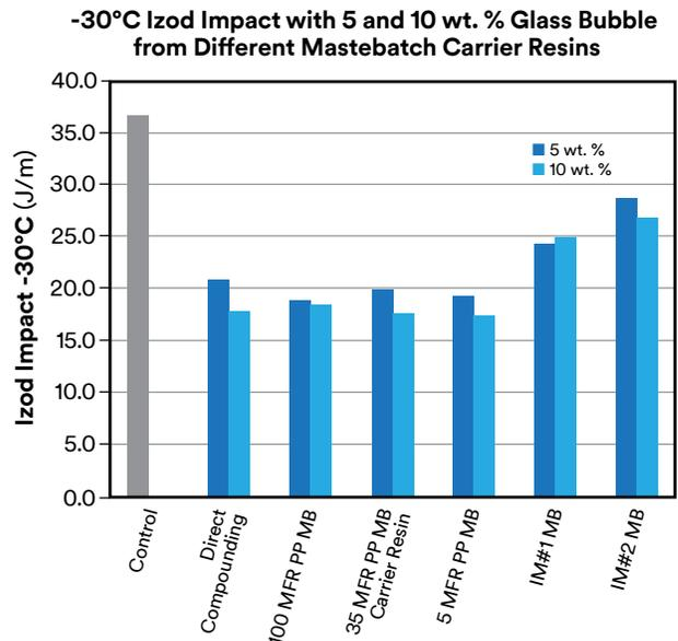
Figure 8. -30°C Izod Impact Changes with Different Masterbatch Carrier Resins
