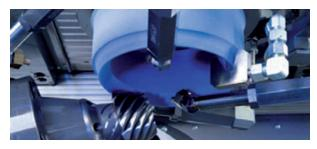
Generation grinding in bevel gear machining is a discontinuous grinding process in which machining is done tooth by tooth. The generating movement of grinding wheel and workpiece is coupled.
