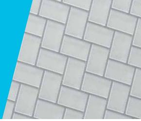
Innovative groove design of the 3M<sup>™</sup> Trizact<sup>™</sup> CMP Pad with independent unit cells — shown here as an optical microscope image.
