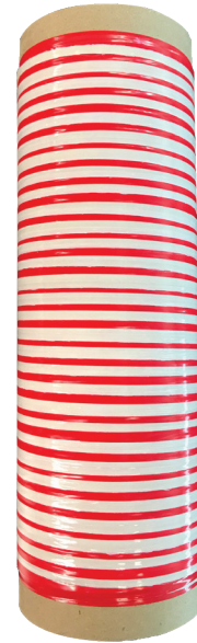
Nextel Towpreg (white) on polyethylene liner (red).
