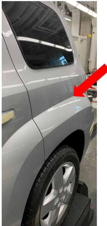
*Figure 1. Rear quarter panel of 2011 Chevy HHR indicating representative location for conformability experiential testing.*
