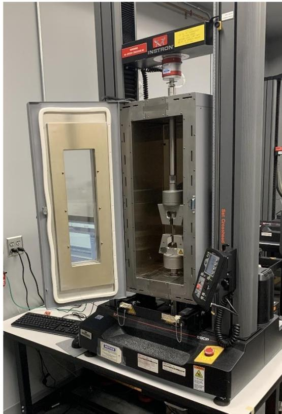
Figure 2. UTM with chamber/oven for testing tensile properties at alternative temperatures.
