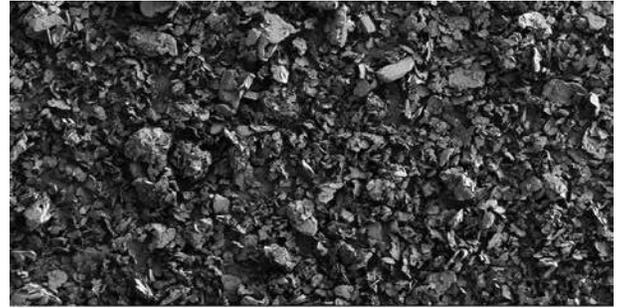
SEM micrograph: Grade CFA50M
