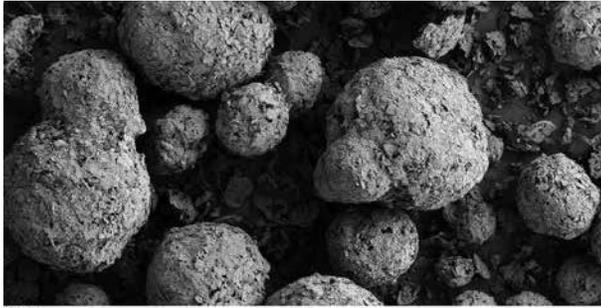
SEM micrograph: Grade CFA250S
