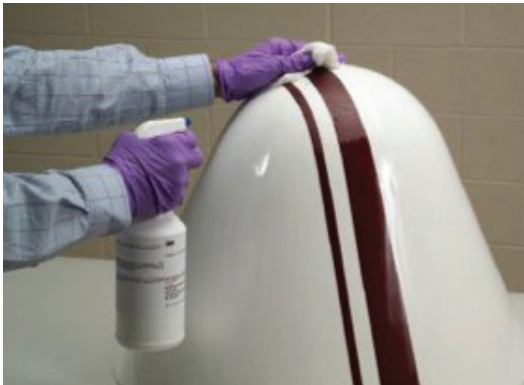
Figure 3: Representative image - Cleaning radome and boot.
