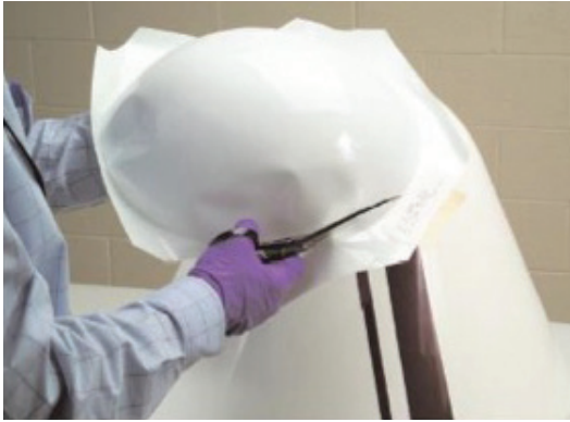
Figure 4: Representative image - Trimming of the boot.
