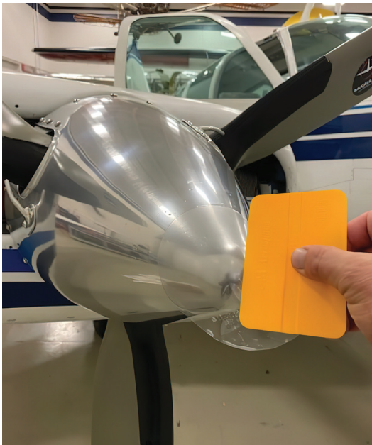
Figure 11: Representative image - Applying and smoothing out boot with the yellow squeegee.
