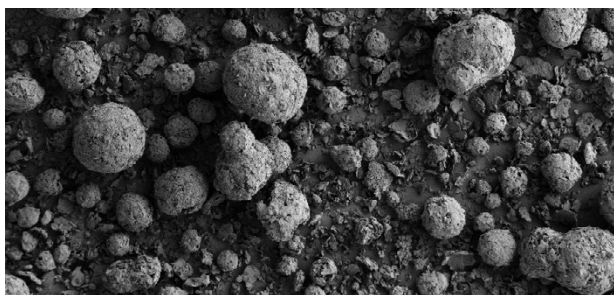
100 µm SEM micrograph: Grade CFA 250S
