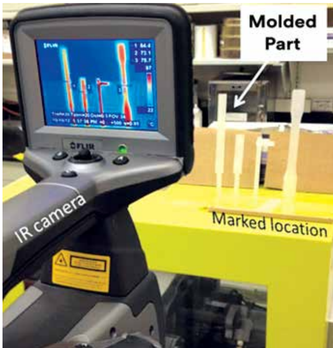
Figure 2. Setup for taking thermal images after part ejection
